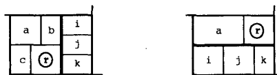
Figure 2: With respect to room r : prime seg (bold line), associated rooms i, j, k , next room i , and Q -state: (r\mathcal{R}\mathcal{R}\mathcal{R}) (left) and (r\mathcal{B}\mathcal{B}\mathcal{B}) (right).
